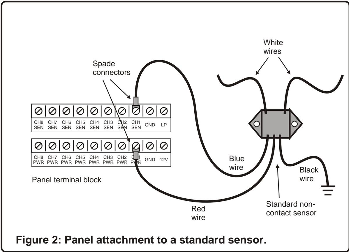
**Figure 2: Panel attachment to a standard sensor.**
