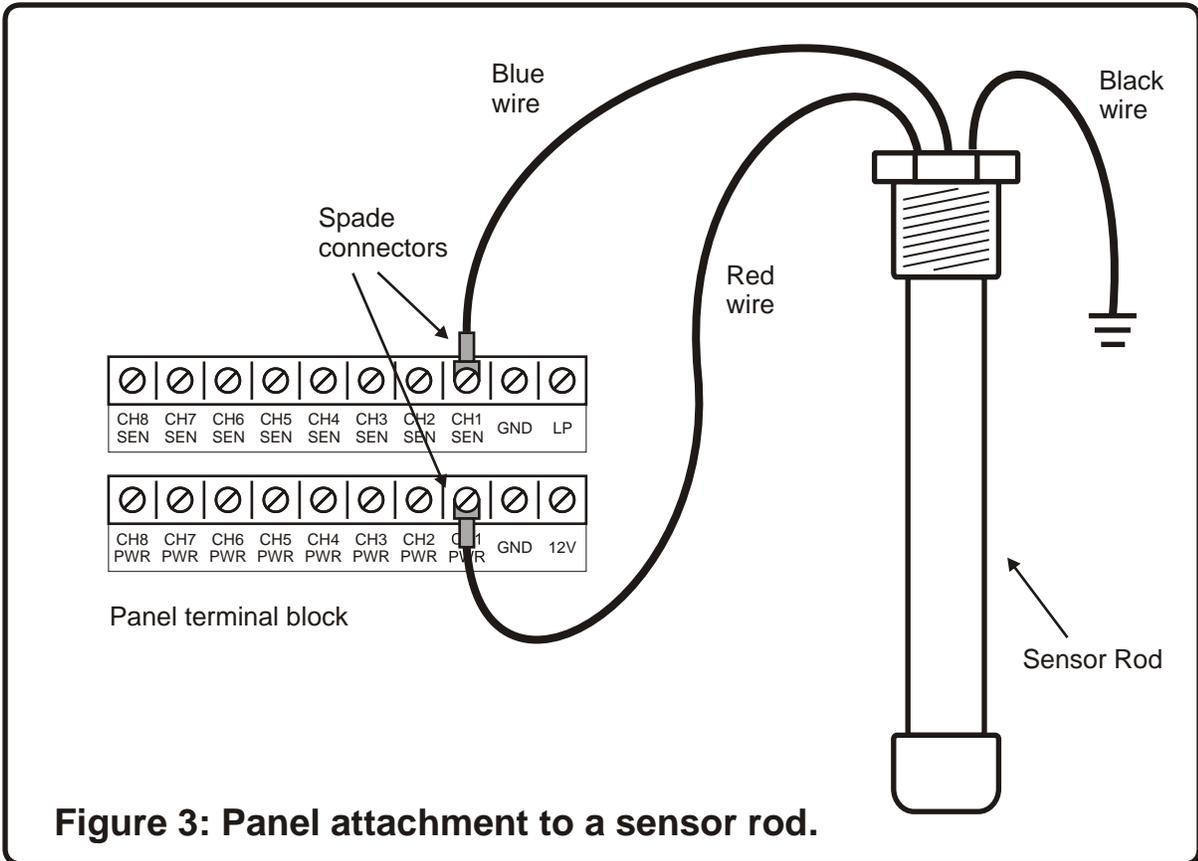
**Figure 3: Panel attachment to a sensor rod.**
