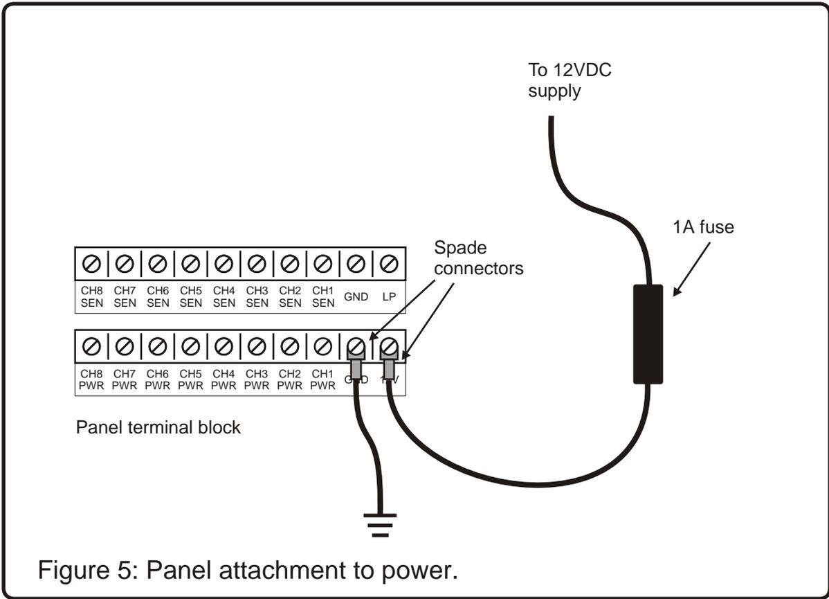
Figure 5: Panel attachment to power.
