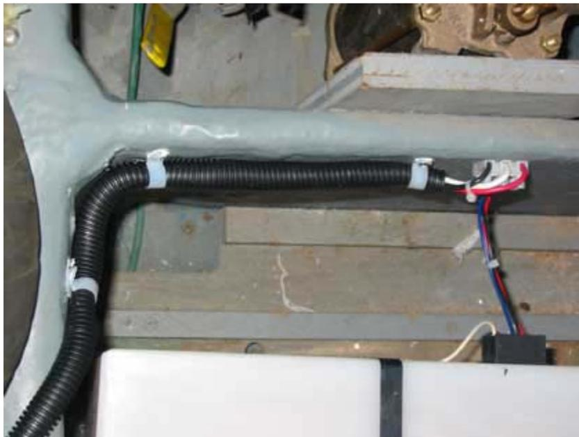
The last foil sensor to be installed was on the Port side water tank. Access to this area proved to be quite difficult, as well as running the wire. Take a break if you have to, and think about the installation for a few minutes. This sometimes brings a solution to light. The fuel tanks were simple; all I had to do is to run a second wire (orange wire at the top) to the existing sending unit. I was assured by the company that this will not result in
