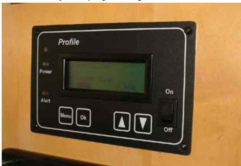
Each sensor channel is configured one at a time. A nifty feature is that there are two labels for each sensor that describes it. For instance, "Waste Tank" can be programmed in for the holding tank. Other configuration parameters include whether to alarm on full, empty, or no alarm at all, sensor type, and tank shape. Tank shape is significant;
