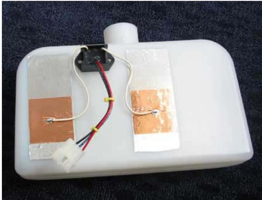
The first item to be done is to clean the area of the sensor installation with alcohol. Then cut two of the supplied aluminum strips to length, one inch shorter than the tank height. The strips are self-adhesive, and are very sticky. It is easy to ruin the strips if you are not careful. When you get the strips cut, remove the backing and place the first strip on the tank so that it is 1/2 in from both top and bottom. The second strip parallels the first - 3 to 4 inches apart.
